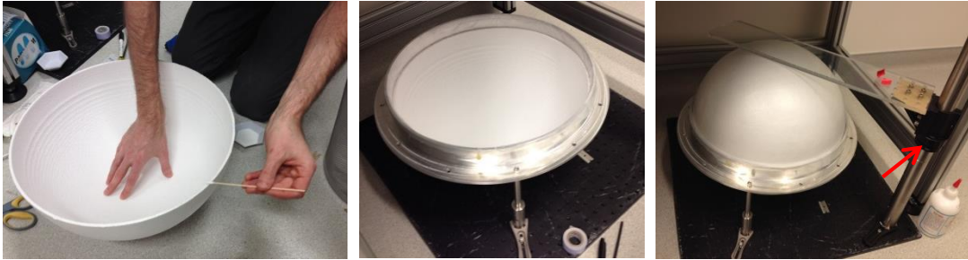
Figure 1.6 Initial gluing of foam sphere.
