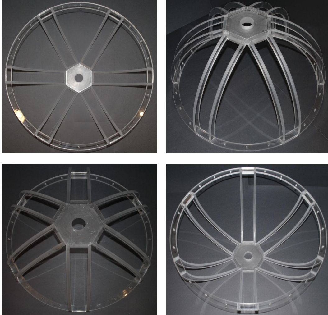
Fig A2. The treadmill frame. All panels, example of a fully assembled 24" treadmill frame See fig A7-9 for parts.
